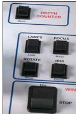
Easy-to-use controls, with adjustable Focus and Iris
